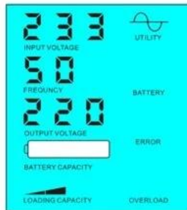
Battery dead, utility supply power
