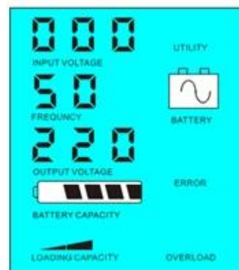
Without utility and battery supply power
