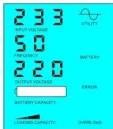
Battery dead, utility supply power
