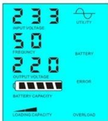
Utility supply power and charge battery
