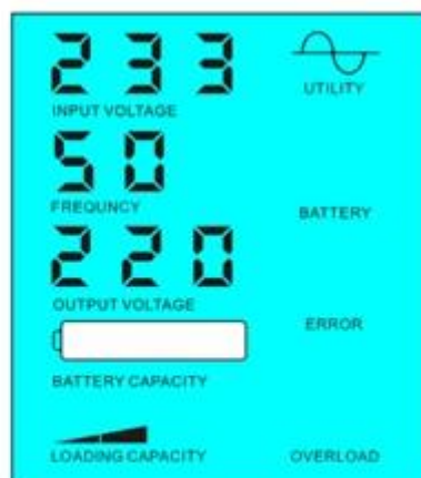
Battery unavailable, utility supply power
