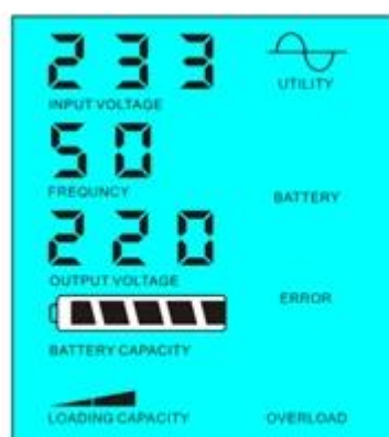
Utility supply power and charge battery
