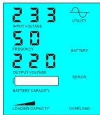
Battery dead, utility supply power
