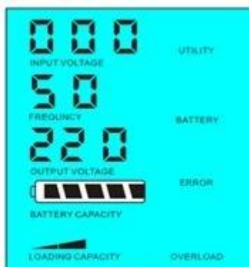
Load's power > 5% of inverter's rated power
