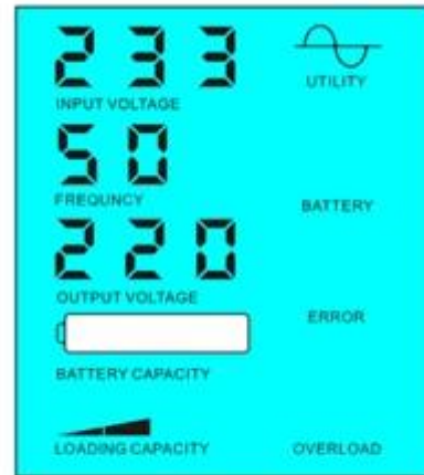
Battery unavailable, utility supply power
