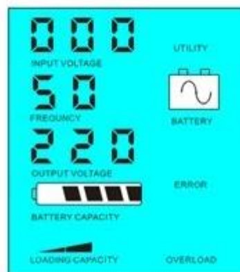
Without utility and battery supply power
