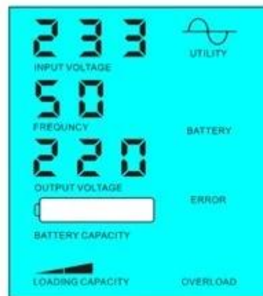
Battery dead, utility supply power
