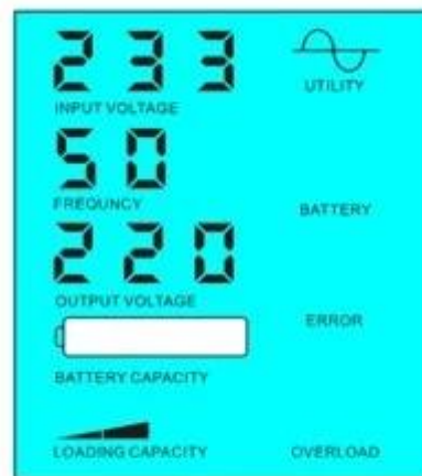
Battery dead, utility supply power
