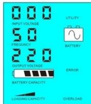
Without utility and battery supply power
