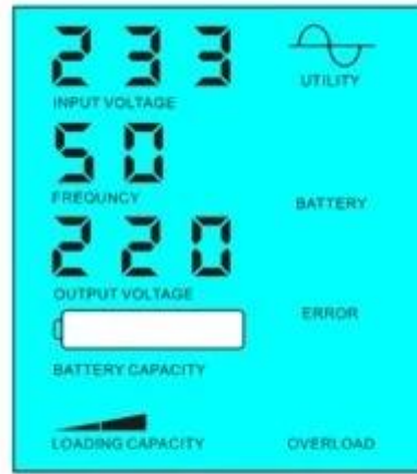
Battery dead, utility supply power
