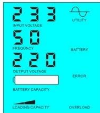
Battery dead, utility supply power
