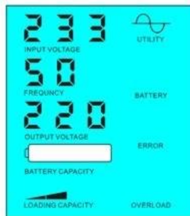
Battery dead, utility supply power
