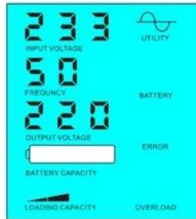
Battery dead, utility supply power
