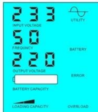
Battery dead, utility supply power
