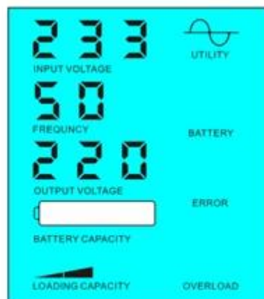
Battery unavailable, utility supply power
