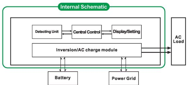
3.1. Utility first battery standby UPS mode (on the panel turn the button to "AC")
