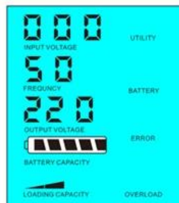
Load's power > 5% of inverter's rated power
