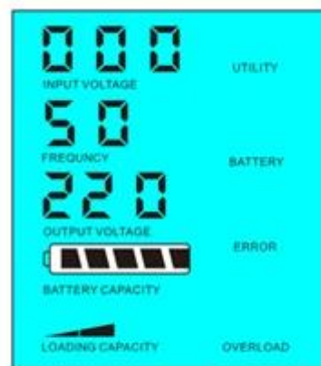
Load's power > 5% of inverter's rated power
