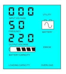
1.2[Sleep mode]FREQUNCYin the LCD display is set as 02.If the power of the connected AC loads is lowerthan 5% of the inverter's rated power, there will be no output from theinverter. Only the chip of inverter is working. The powerconsumption of the inverter is only 1-6W. The LCD shows the output voltage 0. If the power of the connected loads is over 5%, then the inverter willautomatically convert DC to AC to supply power for the loads within 5s. The LCDshows the output voltage. As shown below:
