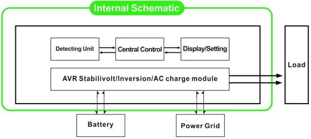
2.1 Utility first (AC first) batterystandby mode : FREQUENCY in the LCD display is set to 01. When utility and batteryare connected to the inverter, utility will supply power to theloads prior. When utility is cut off, the battery will automatically continue supply power via power inverter.
