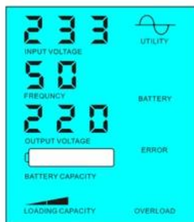
Battery unavailable, utility supply power
