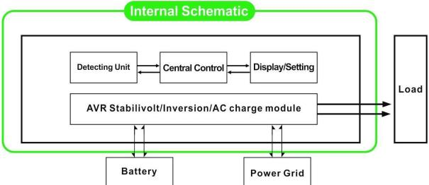
2.1 Utility first (AC first) battery standby mode : FREQUENCY in the LCD display is set to 01. When utility and battery are connected to the inverter, utility will supply power to the loads prior. When utility is cut off,
