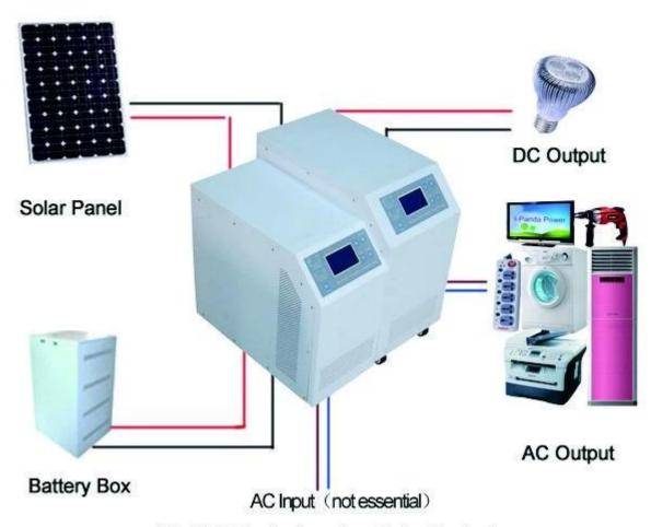
I-P-HPC-Series Inverter+Solar Controller
