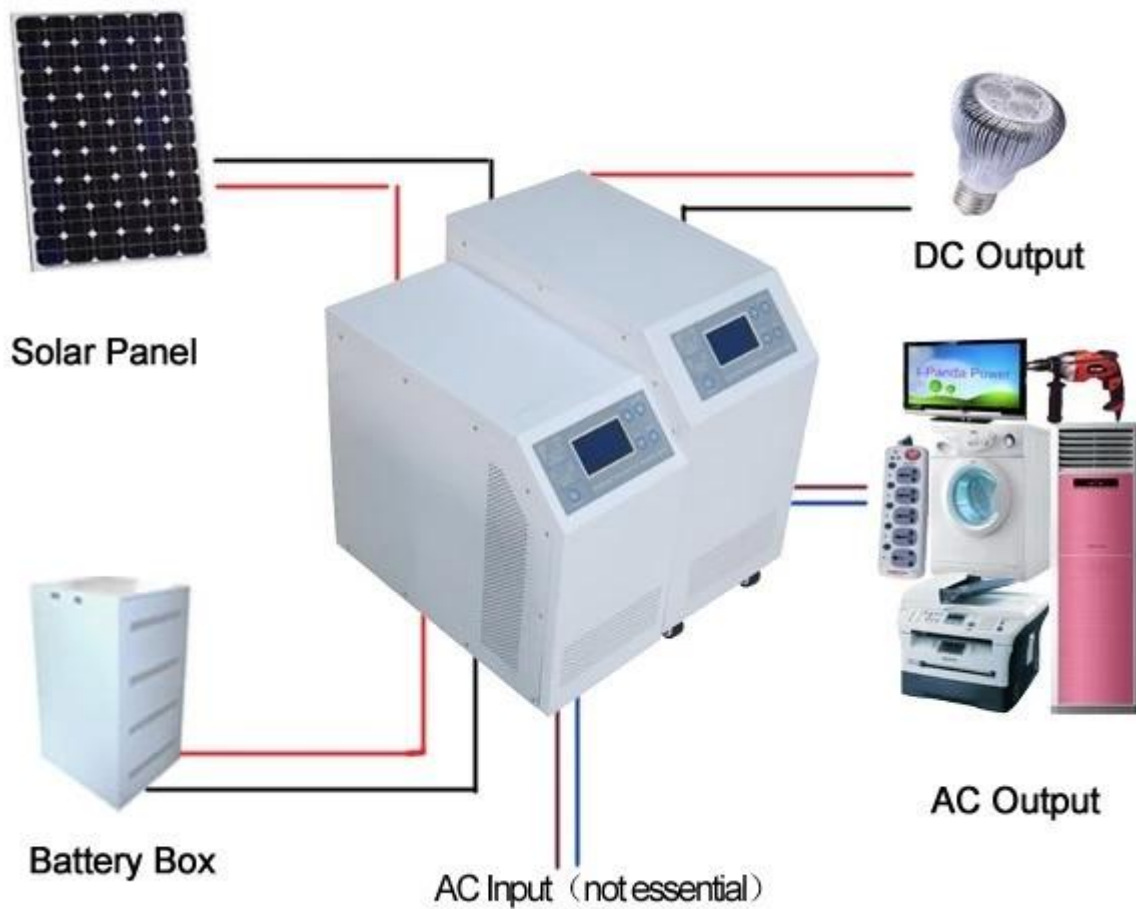
I-P-HPC-Series Inverter+MPPT Solar Controller
