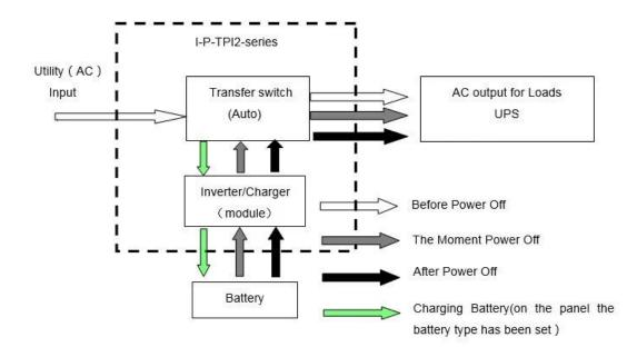
3.2. Battery first utility standby UPS mode (on the panel turn the button to "DC").
