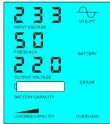
Battery dead, utility supply power
