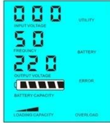
Load's power > 5% of inverter's rated power
