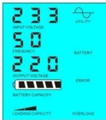
Utility supply power and charge battery
