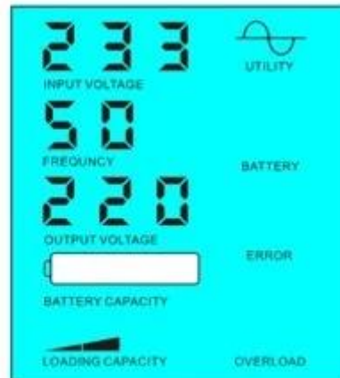
Battery dead, utility supply power
