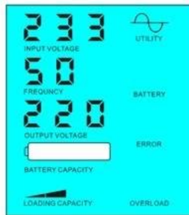
Battery dead, utility supply power
