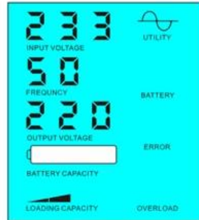
Battery unavailable, utility supply power
