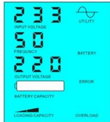
Battery unavailable, utility supply power
