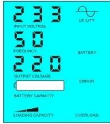
Battery dead, utility supply power
