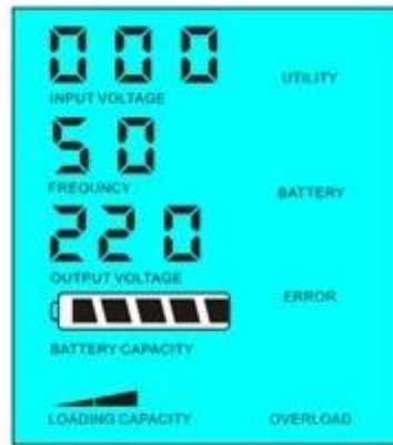
Load's power > 5% of inverter's rated power
