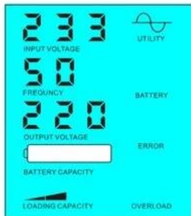
Battery dead, utility supply power
