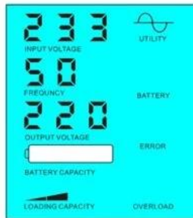
Battery dead, utility supply power
