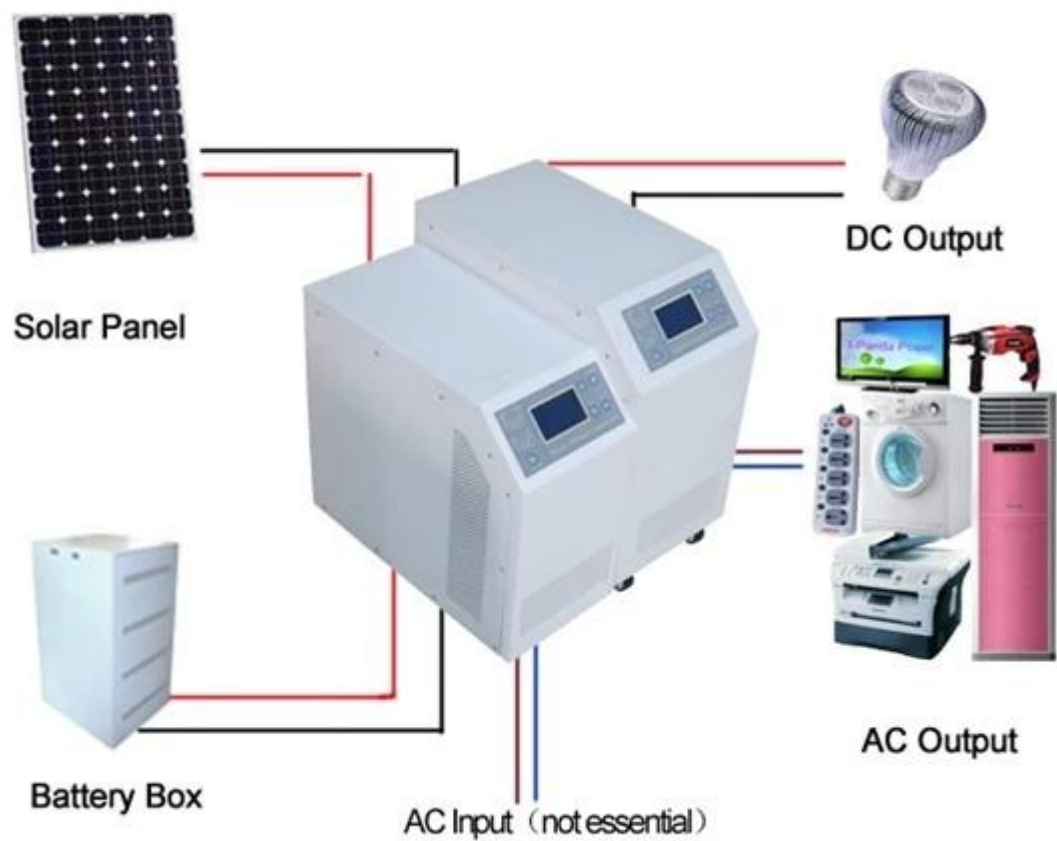
I-P-HPC-Series Inverter+MPPT Solar Controller
