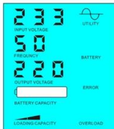
Battery unavailable, utility supply power
