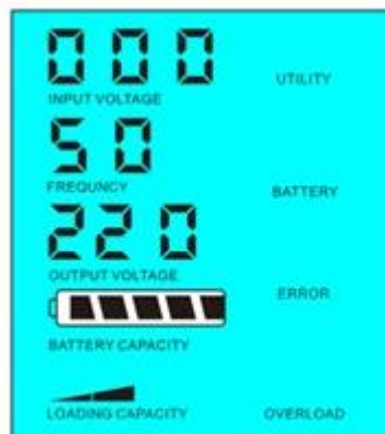
Load's power > 5% of inverter's rated power
