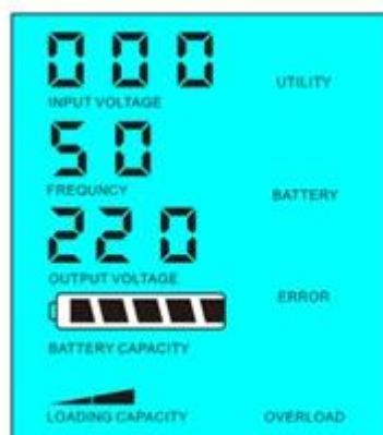
Load's power > 5% of inverter's rated power
