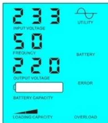
Battery dead, utility supply power
