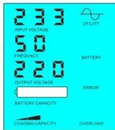
Battery dead, utility supply power
