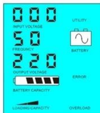
Without utility and battery supply power
