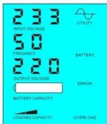
Battery dead, utility supply power
