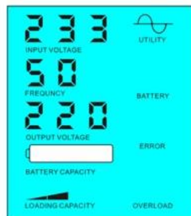
Battery unavailable, utility supply power
