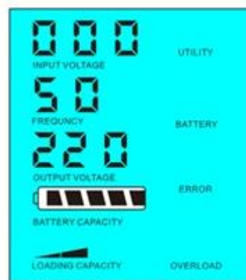
Load's power > 5% of inverter's rated power
