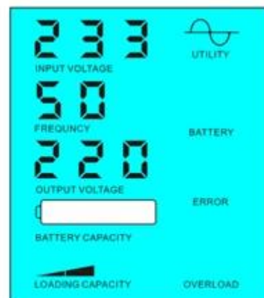
Battery unavailable, utility supply power
