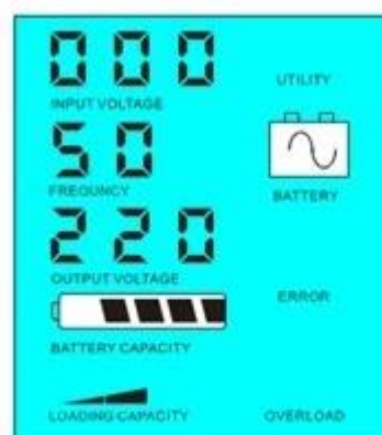
Without utility and battery supply power
