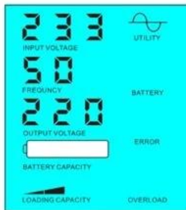
Battery dead, utility supply power
