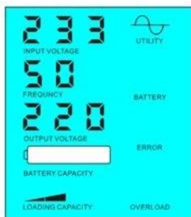
Battery dead, utility supply power
