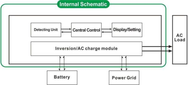
3.1. Utility first, battery standby UPS mode (on the panel turn the button to "AC")3.2. Battery first, utility standby UPS mode (on the panel turn the button to "DC").
