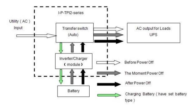
3.2. Battery first, utility standby UPS mode (press the button to "DC").
