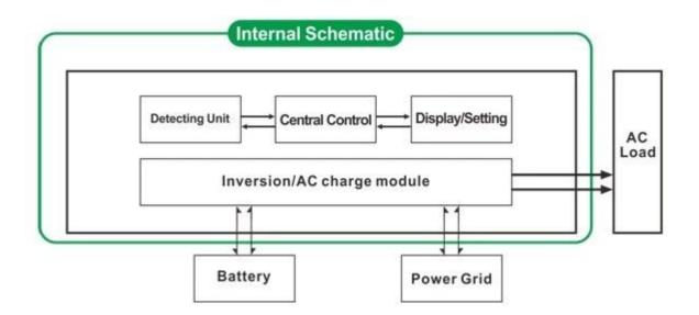
3.1. Utility first, battery standby UPS mode (press the button to "AC")
