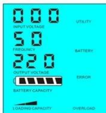
Load's power > 5% of inverter's rated power
