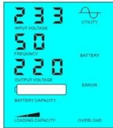
Battery dead, utility supply power
